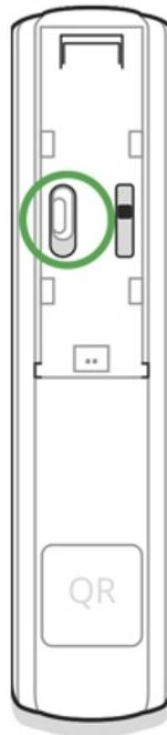
For detection and pairing to occur, the detector should be located within the coverage area of the wireless network of the hub (at a single protected object). The connection request is transmitted for a short time: at the moment of switching on the device.
