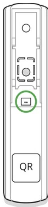
We recommend installing the wired detector at a distance no longer than 1 meter to GlassProtect. Longer wire length increases the risk of its damage and reduces the quality of communication between the detectors.
